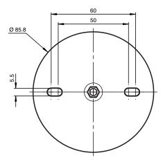
Screw the device onto a level mounting surface using two M5 attachment screws. The attachement screws are not included. Screw a blind plug onto spare connections to ensure the protection category.
