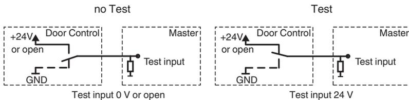
If the device is not used as a safety sensor in accordance with DIN 18650, there is no need to connect the test input.
