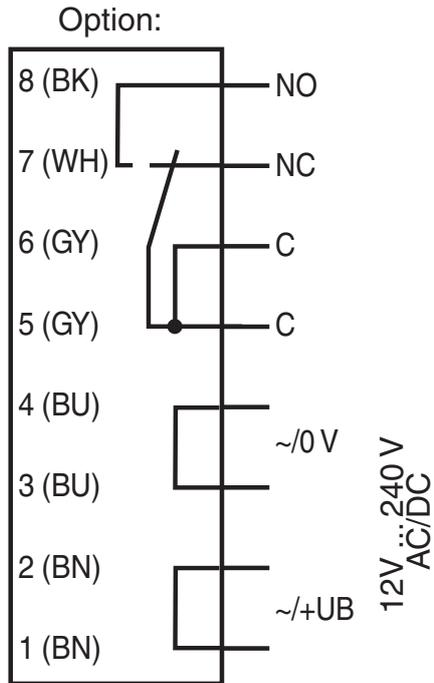
The relay-functions "NC" and "NO" bear on the switching mode "Light-ON". This complies to the default setting of the light/dark switch, located on top of the housing (factory setting).
