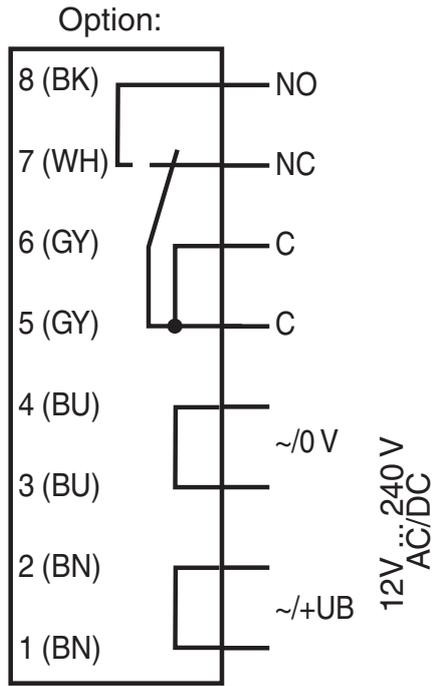
The relay-functions "NC" and "NO" bear on the switching mode "Dark-ON". This complies to the default setting of the light/dark switch (factory setting).
