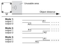
A1  $\longrightarrow \infty$ , A2  $\longrightarrow \infty$ : Object presence detection. Both outputs operate according to the selected mode, if an object is located within the detection range.
