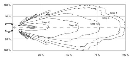
Sensitivity adjustment for suppression of disturbing targets Remove the actual target object from the detection range.
