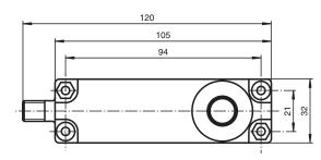
Bore hole and countersinking for screws/hexagon M4
