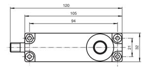
Bore hole and countersinking for screws/hexagon M4
