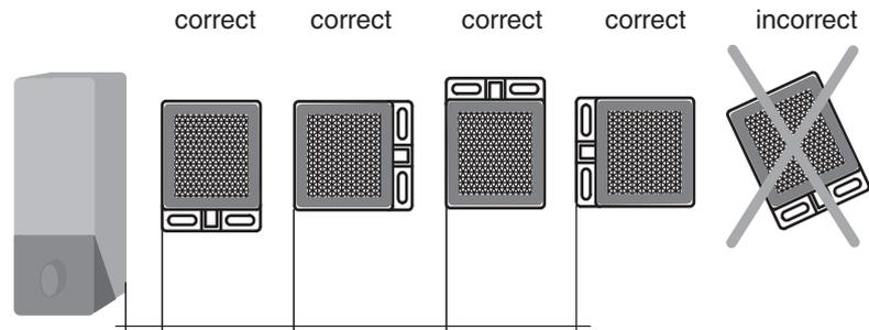
The edge of the sensor must be parallel with the edge of the reflector !
