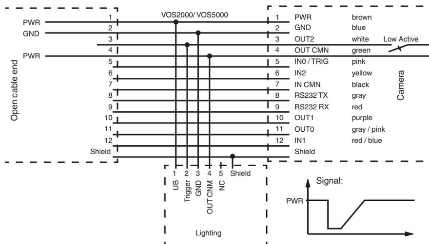
**NOTE:** With trigger parameterization by means of software, the electrical status of the trigger is output to the outside at GPO2 (OUT2). Isolation recommended.
