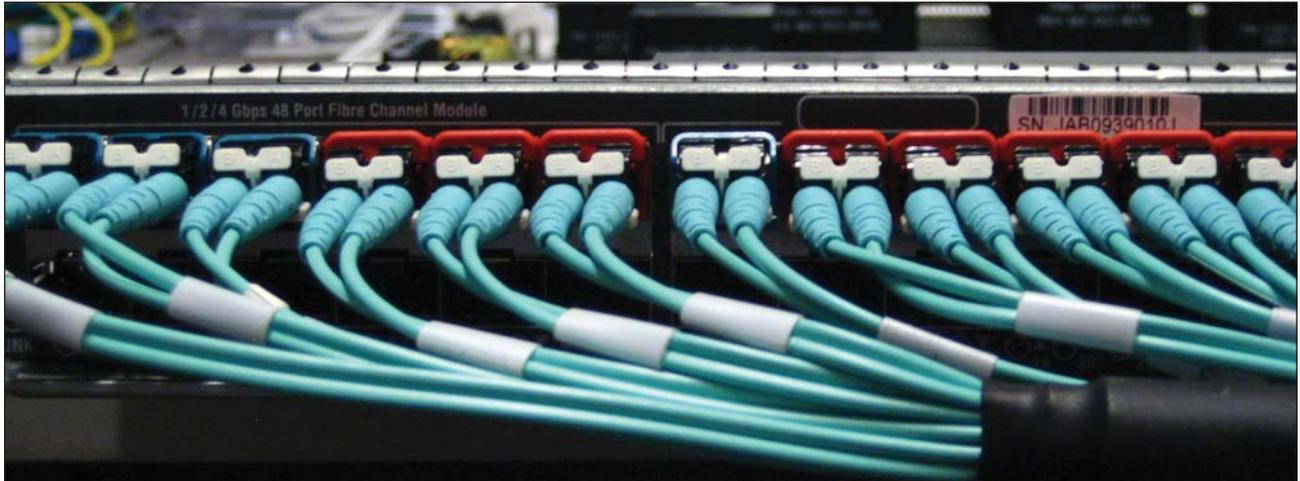
**Figure 4.** Fiber Switch Blade utilizing the LCTRDC
