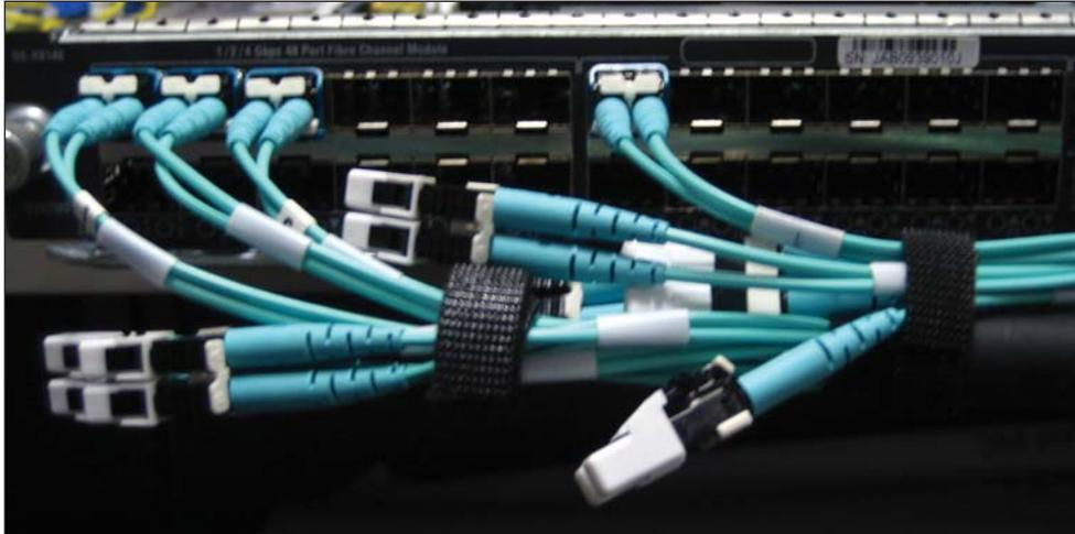
**Figure 1.** Fiber Switch Blade not utilizing all LC connectors on the hydra cable
