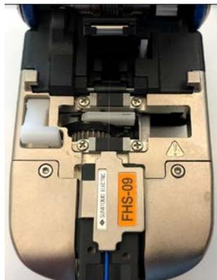
*Figure 8: The stripped and cleaned field fiber in the 900um holder, set into the cleaver.*
