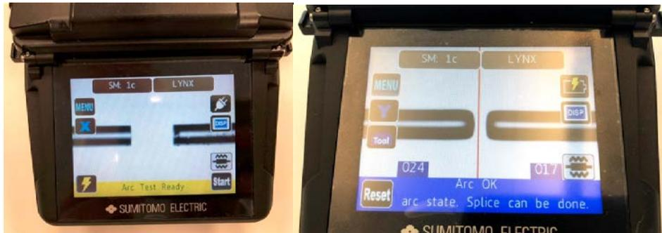
Figure 9: Arc Test before (left) and after (right)
