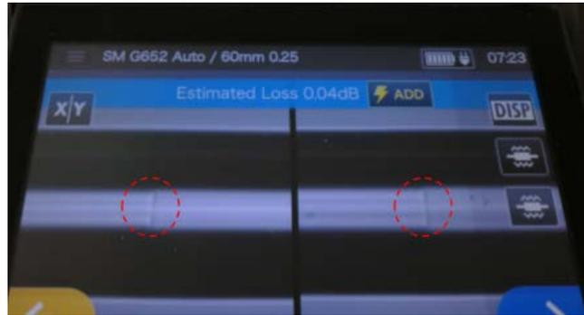
Figure 5: G.652 singlemode fiber spliced to G.657.A2/B2 glass. Note the apparent difference in cores and defined splice event.
