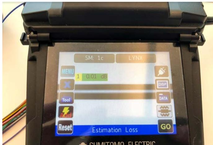
Figure 7: The splice machine estimates the loss of this particular splice to be 0.01dB IL, which is included in the overall loss of the connector.
