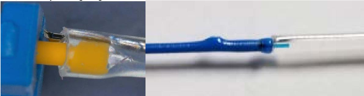
Figure 6: Examples of incorrect heat settings - Overshrinking the shrink tube resulting in the strengthening rod protruding and potentially damaging other components (left); Blistering and charring of the buffer (right).
