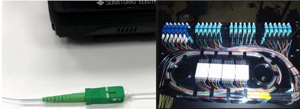
Figure 1: A splice-on connector on 250um cable (left) and a fiber splicing solution (right).
