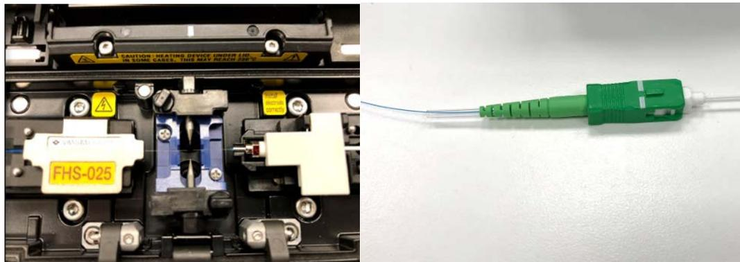
Figure 2: Field fiber being spliced to the connector ferrule (left) and the assembled connector (right).
