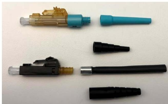
Figure 4: A mechanical splice OptiCam® connector (top) and the components of a field-polish connector (bottom).
