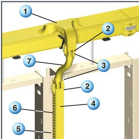
Another option is to use flexible corrugated loom tubing from the spill-over fitting to the 2x2 slotted hinged duct. This approach eliminates the time required to position and secure multiple individual fittings to create a protected pathway.
