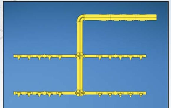
The Distribution and Feeder configuration is the basic, economic layout used to route cables out of the MDA. A higher capacity Distribution Run is used to supply the feeders that route cables out to the cabinets in the EDA. The Feeders in turn are positioned over the cabinet line ups to create a pathway that will provide efficient transitions to the vertical cable management areas of the cabinets and not interfere with Cold Aisle cooling air flow.
