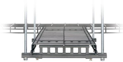
Trapeze brackets are supplied with integral slide clips for securing the pathway in place, eliminating loose hardware. In addition, trapeze bracket design allows side to side pathway positioning increasing installation adjustability.
