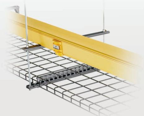
Brackets allow FiberRunner® 4x4, 6x4, 12x4, and 24x4 Pathways to be supported at any height above or below the Wyr-Grid® System. This installation utilizes the same threaded rod to support both systems.
