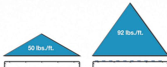
In a high density application a fully loaded 24" wide Wyr-Grid® Pathway will need to support 50 lbs./ft. of cable.
