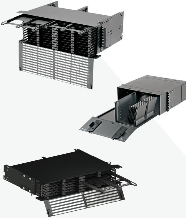
**Enclosures/Panels** – Drawers slide out into locked positions for easy MACs, and house cassettes and FAPs, trunks, connectors, and patch cords. Available in 1-RU, 2-RU, and 4-RU, supporting 144 fibers per rack unit, and can be reconfigured to accept 6-port or 12-port, cassettes or adapter panels.
