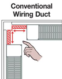
Need for cover access moves conventional duct outward.
