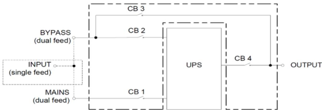
**Figure 8: High-level Maintenance Bypass Switch Block Diagram**
