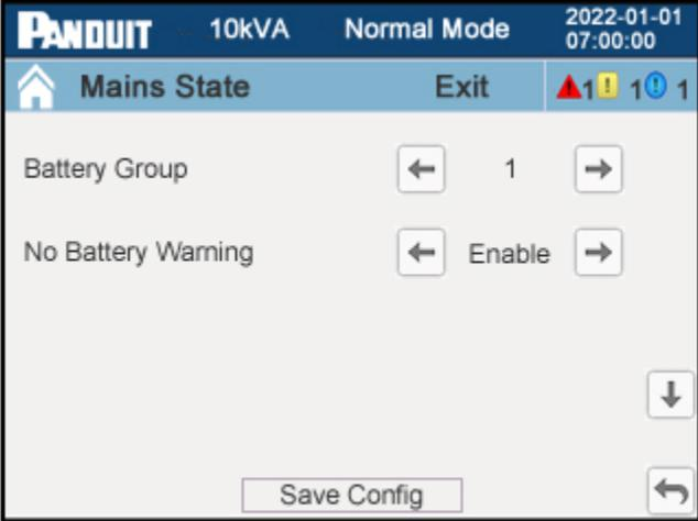
**Figure 46: Battery Setup Page 1 (Single-Phase UPS)**
