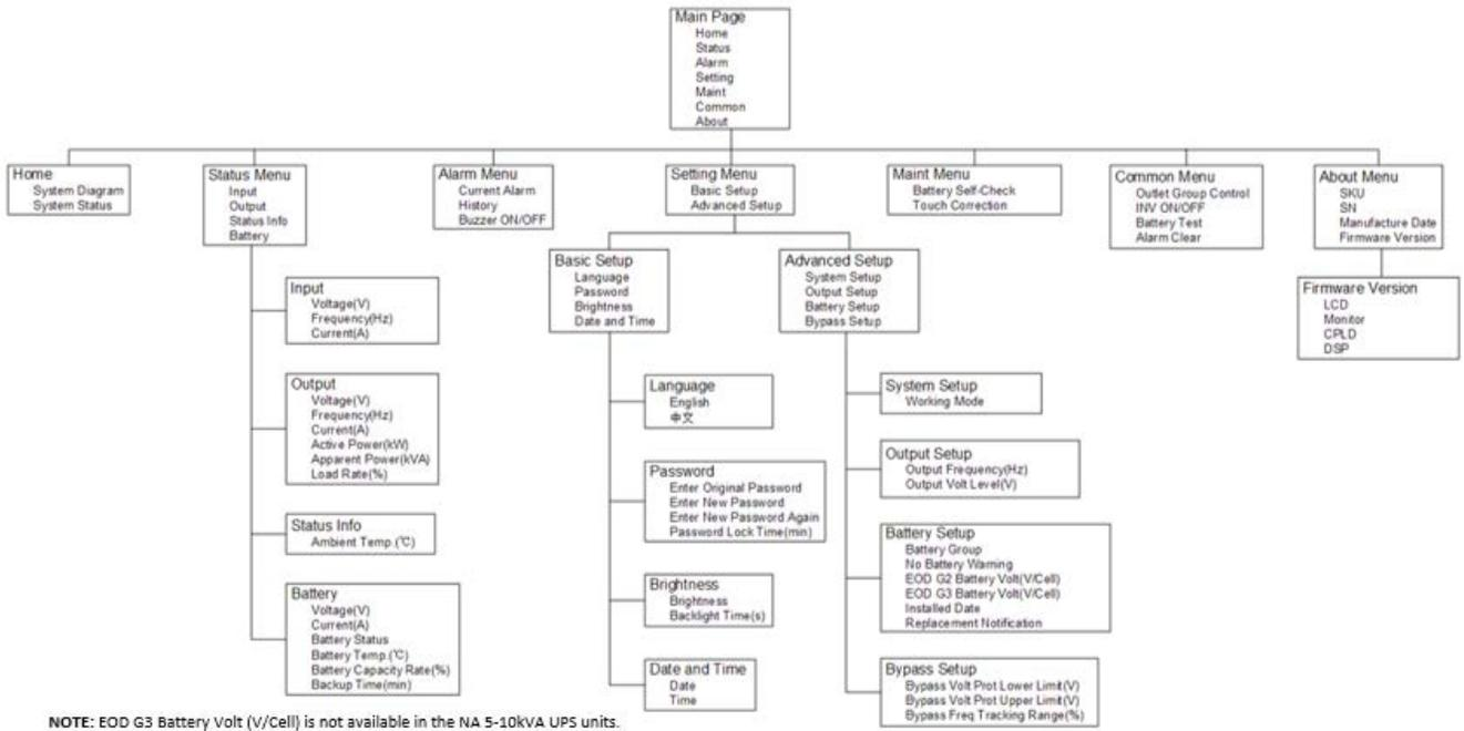
Figure 12: 5-10kVA Single-phase UPS Menu Structure
