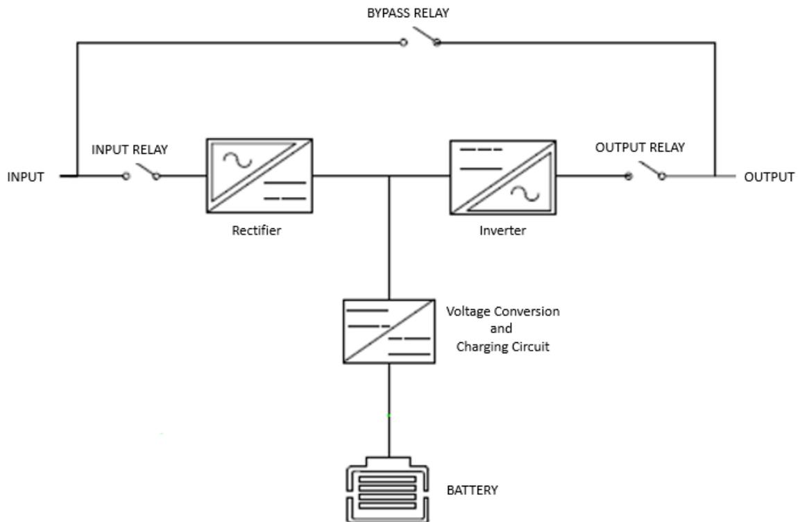
**Figure 1: High-level Generic Double Conversion UPS Block Diagram**
