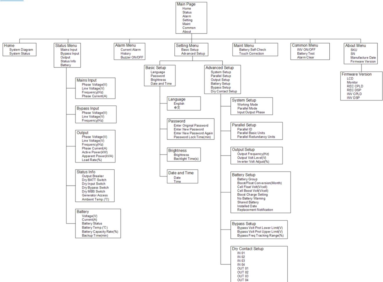
Figure 13: 10 – 20kVA 3-Phase UPS Menu Structure
