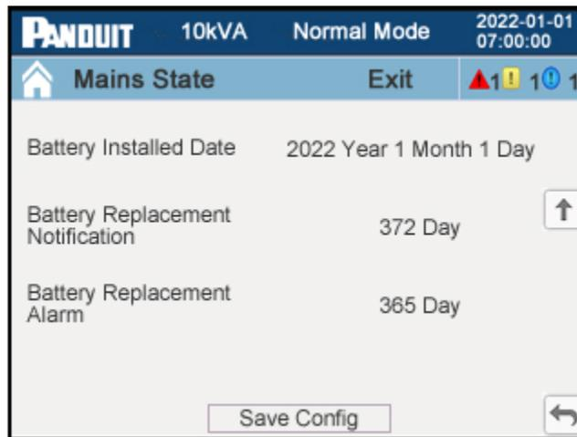
**Figure 48: Battery Setup Page 3 (Single-Phase UPS)**
