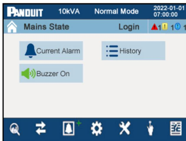
**Figure 29: Alarm Menu Page with Audio ON**
