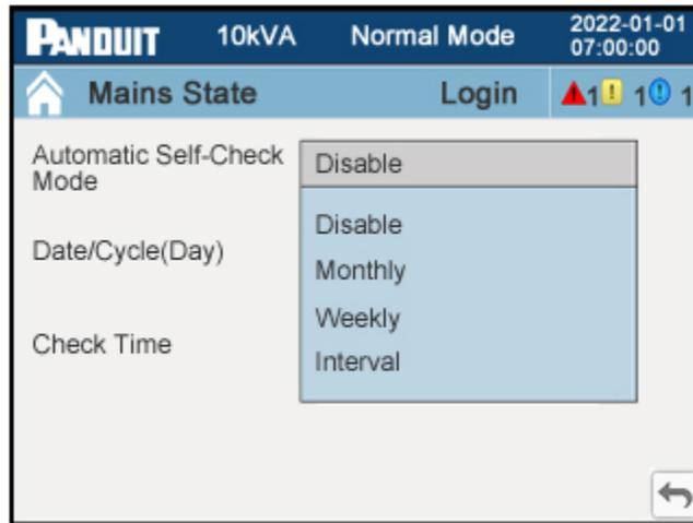
**Figure 56: Battery Self-Check Setup Page 1**
