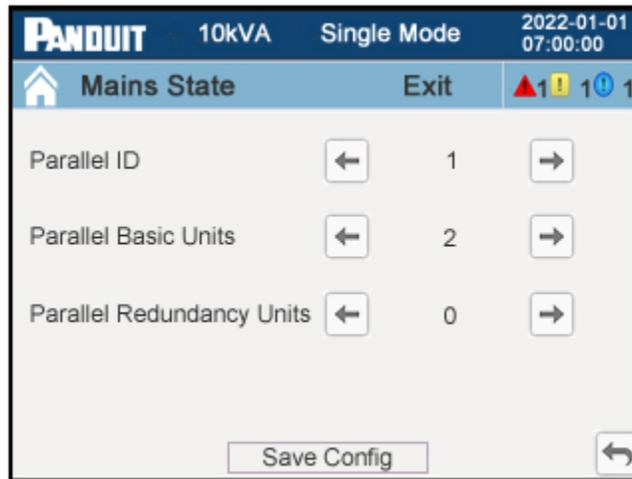
**Figure 44: Parallel Mode System Setup Page (3-Phase UPS)**
