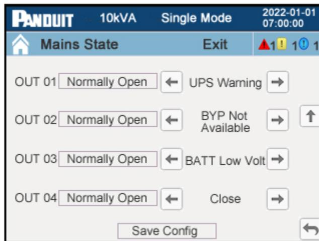
**Figure 54: Dry Contact Setup Page 2 (3-Phase UPS)**
