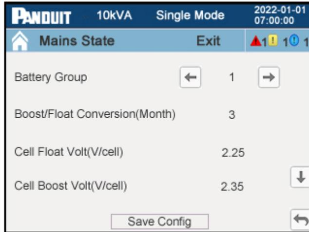
**Figure 49: Battery Setup Page 1 (3-Phase UPS)**
