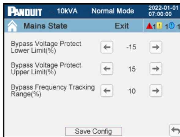
**Figure 52: Bypass Setup Page**
