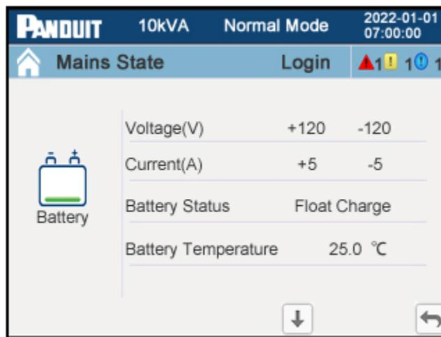
**Figure 27: Battery Status Page 1 (Single-Phase UPS)**
