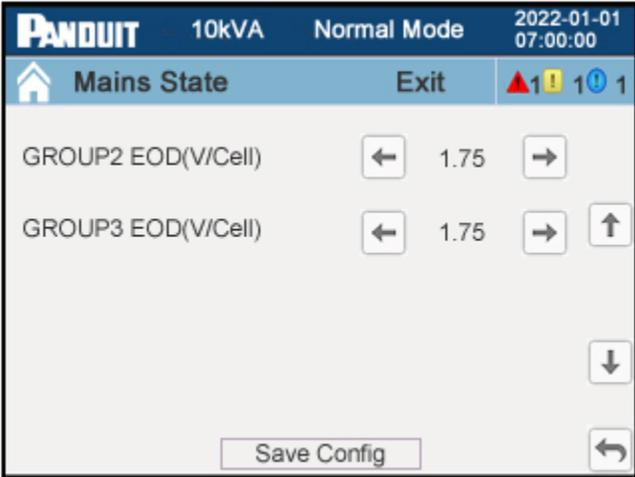
**Figure 47: Battery Setup Page 2 (Single-Phase EU UPS)**
