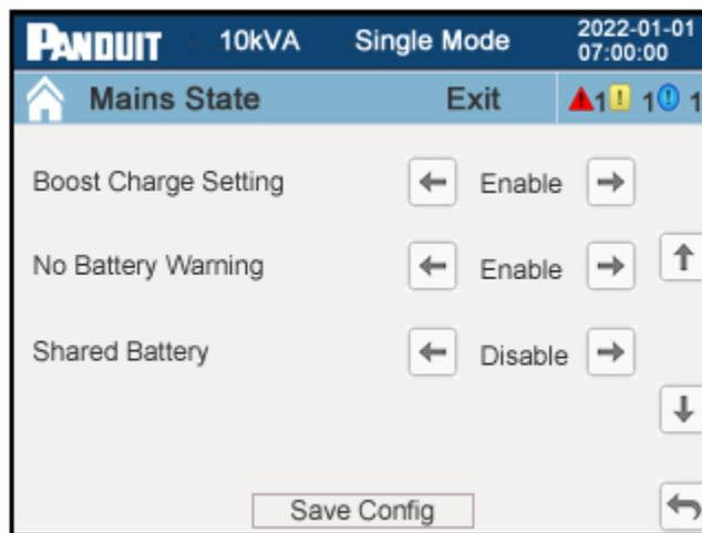
**Figure 50: Battery Setup Page 2 (3-Phase UPS)**
