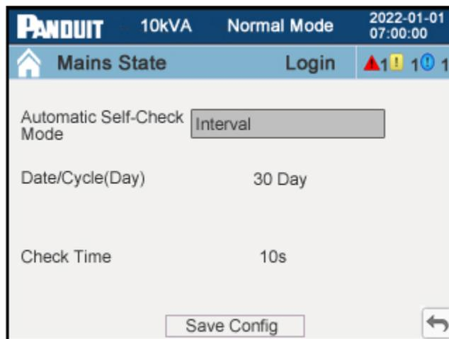
**Figure 60: Auto Self-Check Interval Setup Page**
