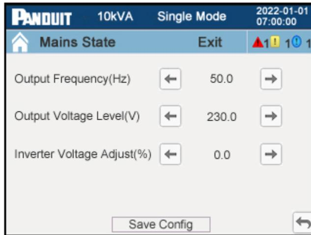
**Figure 45: Output Setup Page (3-Phase UPS)**
