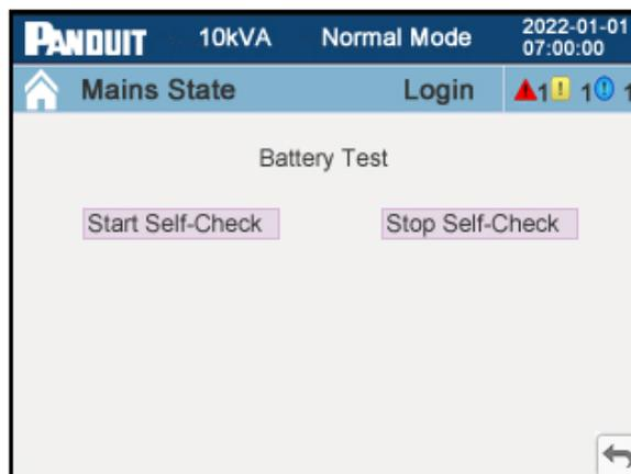
**Figure 65: Battery Manual Test Page**
