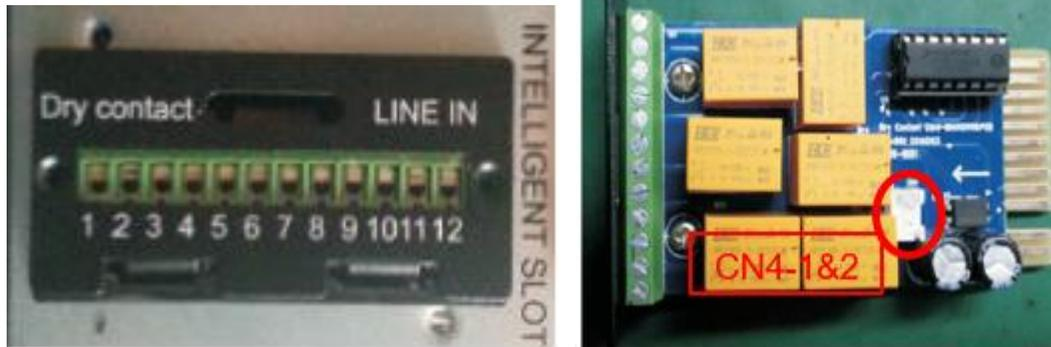
**Figure 16: Relay Card Front and Top View (showing connection points)**
