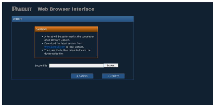
The firmware file should be downloaded and placed on an accessible network drive. After the “image.bin” file is located and the UPDATE button is clicked, the PLA SYSTEM will import and update its software using the new image. After performing a firmware update, the user should immediately cycle the power.
