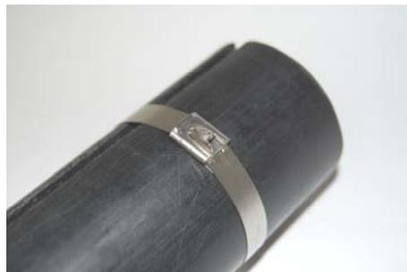
This step completes the tie installation. If installed correctly, the tie should be tight on the bundle.
