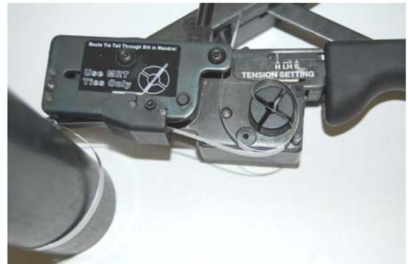
As the tie end is fed through the tool insert the tie end through the Tensioning Split Mandrel. Pull tool tight to bundle.
