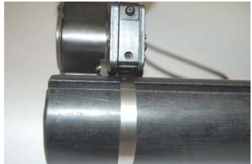
Actuate Tension Handle by squeezing the Tension Handle and Upper Handle together. Continue to do so until the tie is drawn up tight against the bundle. Continue to squeeze the Tension Handle. There will be a noticeable click when the tool has reached the preset tension. The handles will snap together. At this point, the tie is held in the preset tension.
