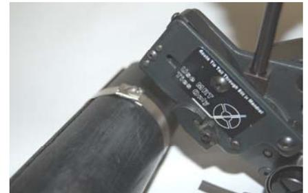
Holding the handles together, grasp the Cutter Handle Lever and move it forward. This action will set ball and cut off the excess tie length flush with the tie head.
