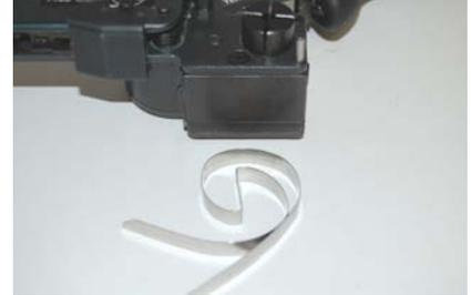
Remove the wound up excess tie length piece.
