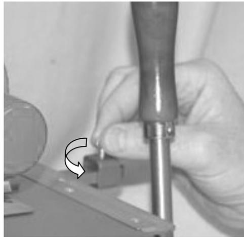
Slide the stop to the right hand end of the stop bar and tighten the thumbscrew.
