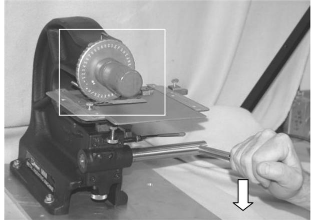
While holding handle down completely, turn screw inward (counter-clockwise) until it stops.
