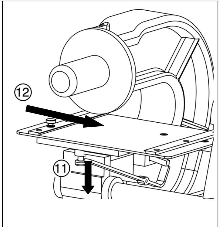
13 Tighten screws securely, in order (after table is placed back onto press).
