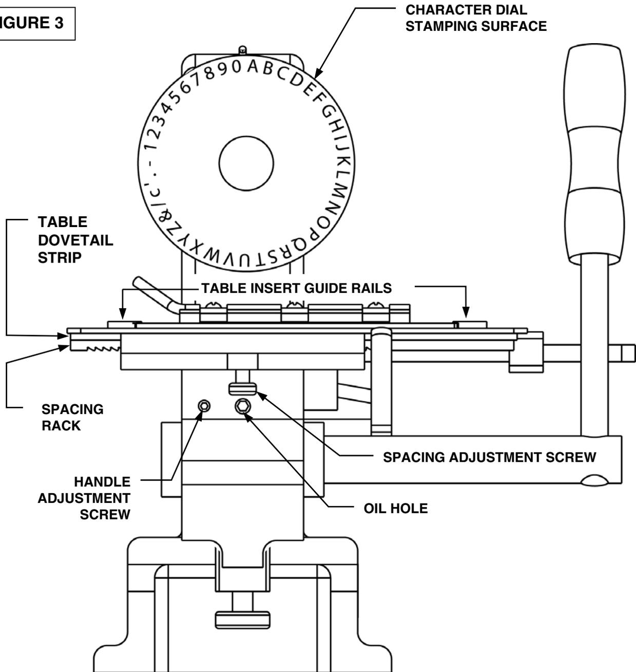
2. Lubricate the rear character dial surface, the table insert guides and the table dovetail strip **with a dry lubricant (graphite type). Do not use oil.**
