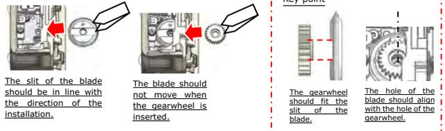
The slit of the blade should be in line with the direction of the installation.
