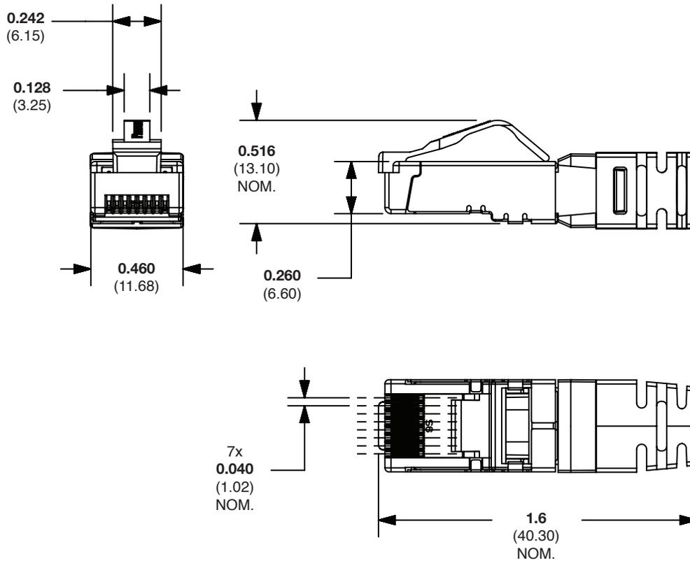
Dimensions are in inches. (Dimensions in parenthesis are metric).
