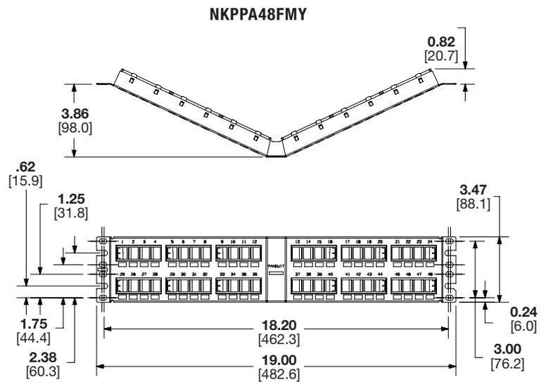
Dimensions are in **inches**. [Dimensions in brackets are metric].
