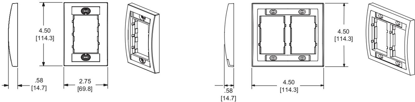
Dimensions are in inches. [Dimensions in brackets are metric].
