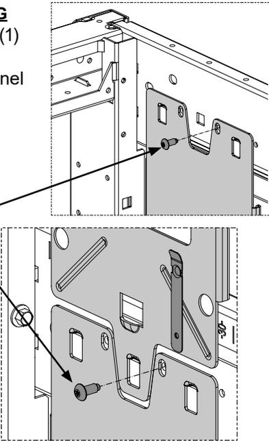
**Moving and Re-installing Vertical Cable Managers**
