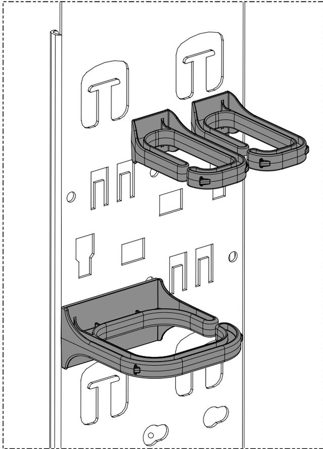
*Install Flex-Clip 18 & L-Rings in orientation shown.
