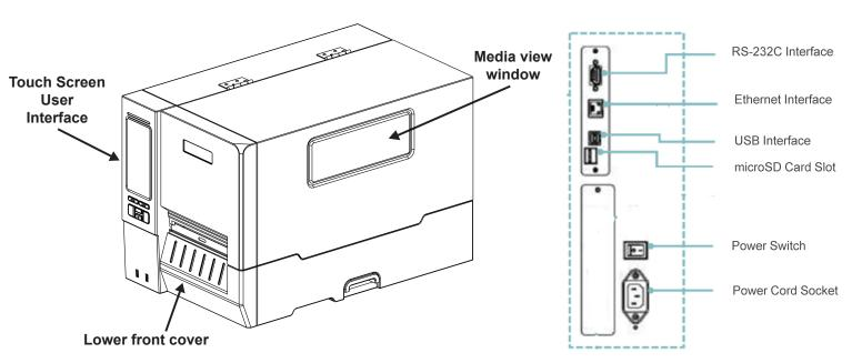
Note: This printer is configured for USB "Plug and Play" installation. For detailed instructions on other installation methods, please review the enclosed User Manual.
