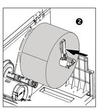
(2) Place the roll of media on the label supply spindle. Flip up the label roll guard. Move the label roll guard horizontally to gently fit the width of label roll.
