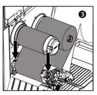
(3) Close the print head mechanism. Push down until you hear a "click" and the print head is engaged.
