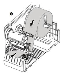
(3) Pull label roll leading edge forward through the media guide bar, damper, media sensor and place the label leading edge onto the platen roller.
