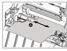
(4) Adjust the gap sensor and place arrows over media gaps.
