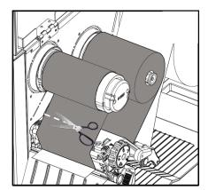
(1) Break the ribbon between ribbon guide plate and the ribbon rewind spindle.
