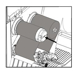
(2) Push the ribbon release button to release the ribbon on the ribbon rewind spindle and remove ribbon.
