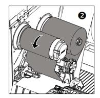
2) Thread the ribbon through the ribbon sensor slot and then through the open space in between print head and platen. Wrap the ribbon onto the ribbon rewind spindle counter clockwise about 3 to 5 circles until smooth.
