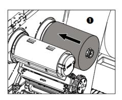
(1) Open the printer right side cover. Slide the ribbon onto the ribbon supply spindle.
