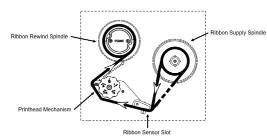
Please note: Panduit ribbon part numbers beginning with RHE must be installed using the inward direction.
