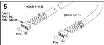
· Orient load bar with contact slots facing downward.
