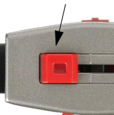
Locking pin is visible (not engaged)
