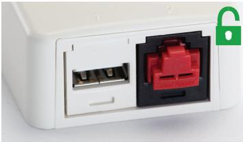
If device is in LOCKED position, use master key to unlock
