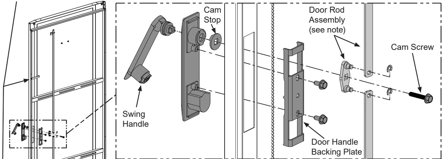
**N-Type Single Hinge Door; N-Type & S-Type Solid Rear Door**
