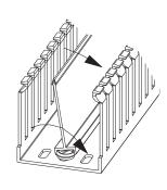
REMOVING FINGERS ON SLOTTED DIVIDER WALL
