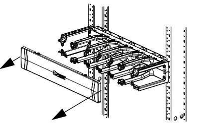
To open the cover downwards, pull out and down on the middle of the cover top. To open cover upwards, pull out and up on the middle of the cover bottom. To remove the cover completely, pull straight out on both ends of the cover simultaneously.
