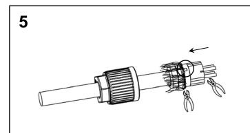
Push splice element onto braid and seal. Trim off excess braid material and cut conductors flush with the splice element.
