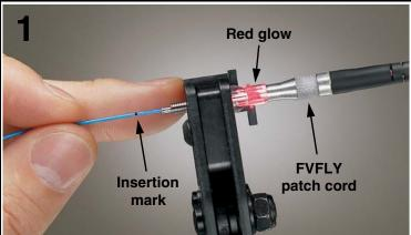
After connecting the FVFLY Fiber Visual Fault Locator to the Opti-Crimp connector ferrule (with the included patch cord), turn the FVFLY "on". Notice the red glow in the connector ferrule. While carefully inserting the cleaved field fiber into the connector using constant light pressure, notice the red glow diminish as the cleaved field fiber approaches the pre-polished fiber stub in the connector. The insertion mark on the fiber will also approach the end of the connector ferrule.
