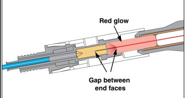
WHY DOES THE FERRULE HAVE A RED GLOW? The red laser light from the FVFLY Fiber Visual Fault Locator will continue to radiate from the end of the pre-polished fiber stub until optimum contact is made between the cleaved field fiber and the pre-polished fiber stub in the connector. As the field fiber approaches the pre-polished fiber stub, less red laser light radiates from the end of the pre-polished fiber stub as it begins to continue through the field fiber.
