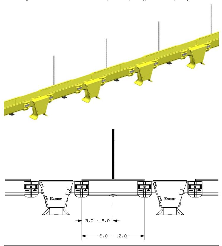
With channel sections over 12" between fittings the placement of a *FIBERRUNNER* Mounting Bracket should be installed 6" from each end of the channel section and at intervals deemed necessary to ensure the integrity of the fiber pathway.
