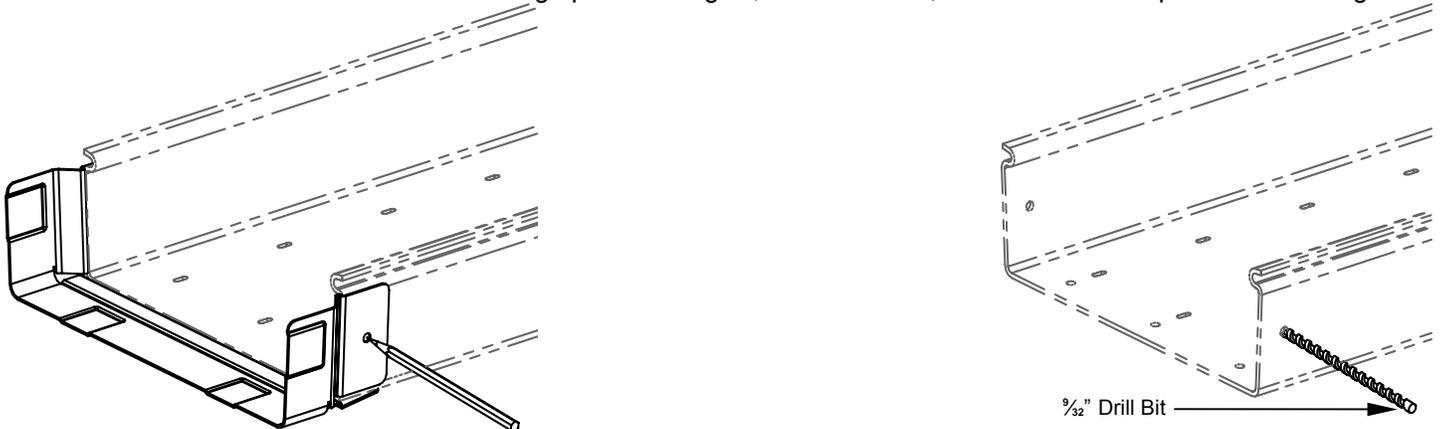
3. Reattach the adapter and realign all five (5) of the mounting holes. With the adapter held in place, insert one (1) of the ¼-20x⅝" Nylon Phillips Binder Head Screws through each of the mounting holes from the inside of the channel. Be sure that all five (5) of the binder head screws are pointing outward away from the adapter. Thread one (1) of the ¼-20 Nylon Deco Wing Nuts on to each of the binder head screws and hand tighten.
