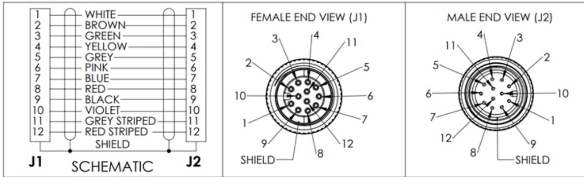
Reader to QX-1 Interconnect Cable – M12 Socket to M12 Plug – 1 Meter, 3 Meters (Right Angle to Back of Camera)
