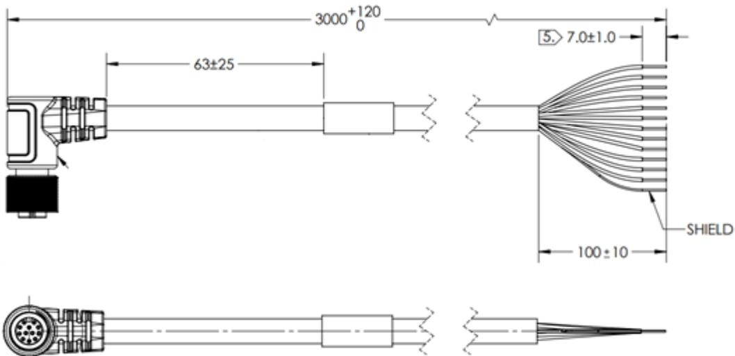
**M12 to Flying Leads Cable – Parallel IO (Power, DIO, RS-232), Right Angle Front – 3 Meters**
