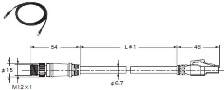
\*1 – Overall cable length varies based on model number. Example: FHV-VNB2 2M is a 2 meter cable.
