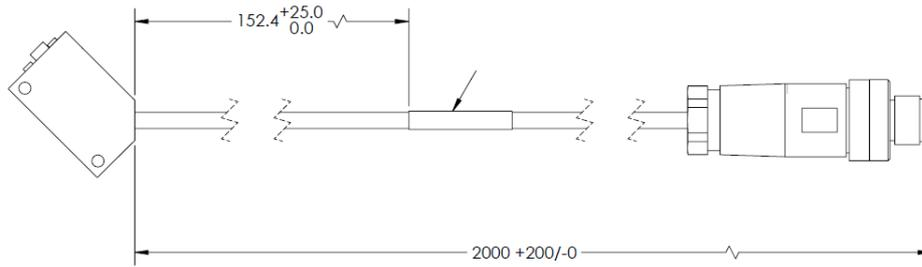
**QX-1 Field-Wireable M12 4-Pin Plug for Any Trigger Source or Photo Sensor – Screw Terminal Connector**
