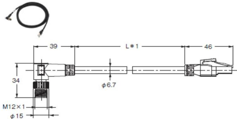
\*1 – Overall cable length varies based on model number. Example: FHV-VNLB2 2M is a 2 meter cable.
