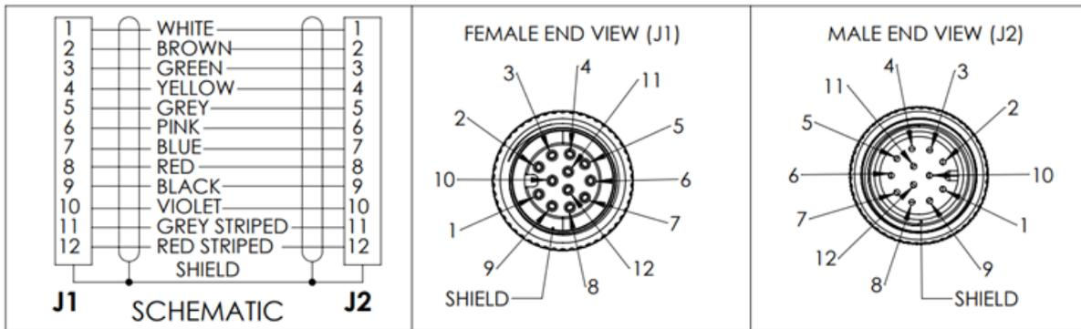
VHV5-F to QX-1 Interconnect Cables with RS-232 Breakout – 3 Meters, 5 Meters
