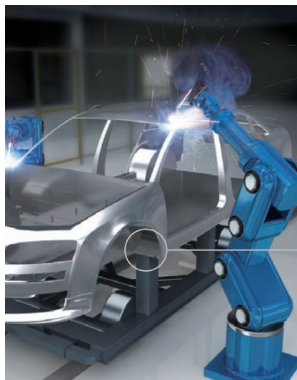
Sitting position check of metal plates to weld
