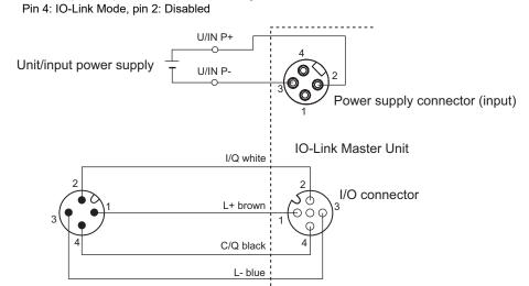
IO-Link device (without digital inputs or outputs for pin 2)
