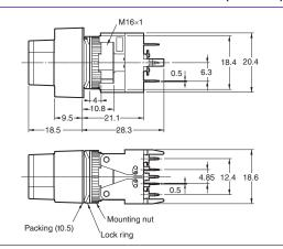
Rectangular A165W□-T Reduced-voltage lighting solder terminals/ tab terminals (#110 t=0.5)
