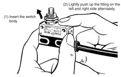
Be sure that the clamp is inserted to the full depth, because the Switch will not function properly if one of the clamps is improperly inserted
