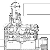
· The bearing load strength has been increased to prevent faulty resetting of the bearing, which may occur when the roller is
