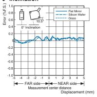
Note: The x-axis displacement indicates the measurement distance displayed by the amplifier unit. The measurement distance displayed by the amplifier unit takes the measurement center distance as 0, and the NEAR and FAR sides from the sensor are displayed by + and -, respectively.
