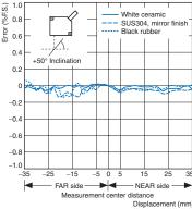
Note: The x-axis displacement indicates the measurement distance displayed by the amplifier unit. The measurement distance displayed by the amplifier unit takes the measurement center distance as 0, and the NEAR and FAR sides from the sensor are displayed by + and -, respectively.
