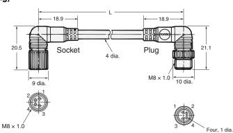
Right-angle (Socket)/Straight (Plug) XS3W-M424-4□□-R (4 poles)
