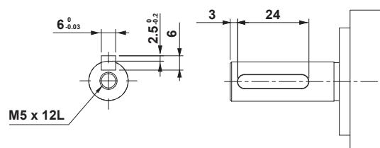
**Type 3000 r/min motors (230 V, 1 kW to 1.5 kW)**
