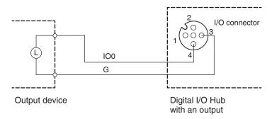
The output power that provides load current is supplied from the IO-Link Master Unit through the IO-Link cable to the Digital I/O Hub.
