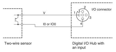
The power to pin 1, or +(V), is supplied from the IO-Link Master Unit through the IO-Link cable to the Digital I/O Hub.
