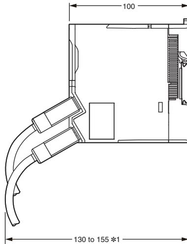
\*1. This is the dimension from the back of the Unit to the communications cables.
