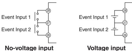
The ON and OFF criteria can be based on the total count of the two inputs, an OR of the two inputs, or the status of the inputs.
