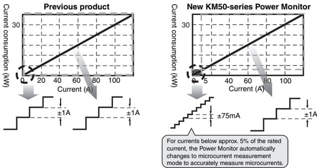
You can measure microcurrents of  $\pm 75$  mA with a CT with a rated current of 100 A. (Reference Value)
