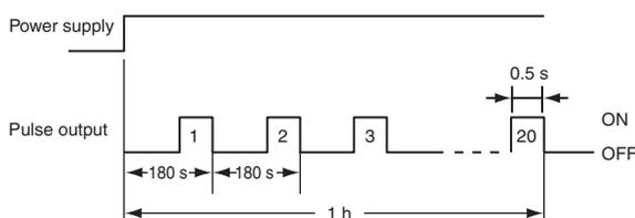
If the cycle becomes shorter than the pulse width or if the output must turn ON immediately after turning OFF, an OFF time of 100 ms will be maintained.
