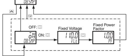
• When the simple measurement function is set to ON, set the fixed voltage value and power factor consecutively.
