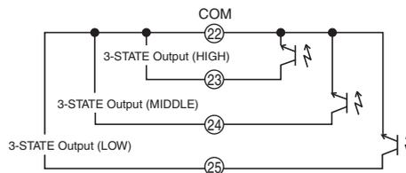
The Three-state Energy Classification of the KM50-E Smart Power Monitor divides the total power consumption into three consumptions, HIGH, MIDDLE, and LOW, based on the user-set HIGH threshold (41.h.th) and LOW threshold (42.l.th).
