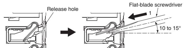
2. With the flat-blade screwdriver still inserted into the release hole, insert the wire into the terminal hole until it strikes the terminal block.
