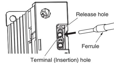
If a wire is difficult to connect because it is too thin, use a flat-blade screwdriver in the same way as when connecting stranded wire.
