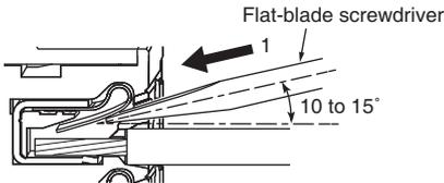
2. With the flat-blade screwdriver still inserted into the release hole, remove the wire from the terminal insertion hole.
