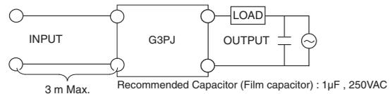
2. The G3PJ with Rated Load Voltage of 100 to 480 VAC (5□□B model)
