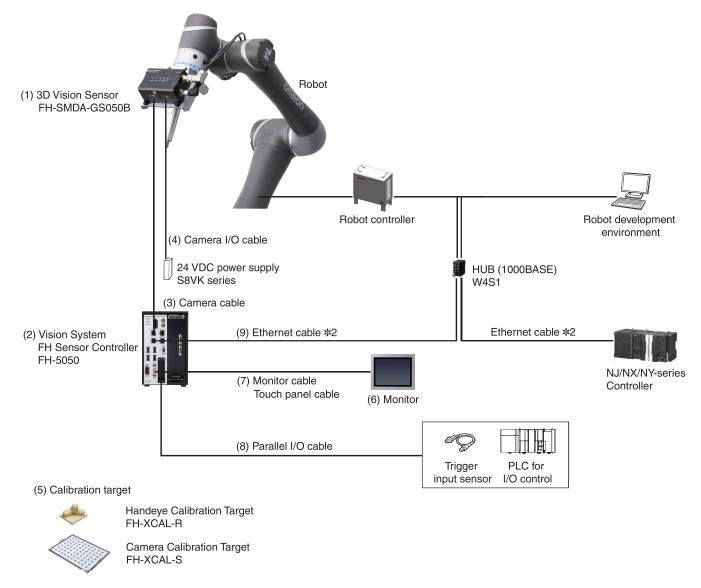
**\*1.** Total time for 3D measurement and 3D recognition under our specified conditions. It varies depending on the target. **\*2.** To use STP (shielded twisted-pair) cable of category 5 or higher for Ethernet and RJ45 connector.
