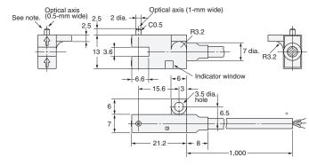
$^{\star}$  Vinyl-insulated round cable of 3.5 dia., 3 cores, (0.14 mm² with 1.0-dia. insulator); Standard length: 1 m  $^{\star}$
