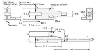
\* Vinyl-insulated round cable of 3.5 dia., 3 cores, (0.14 mm² with 1.0-dia. insulator); Standard length: 1 m
